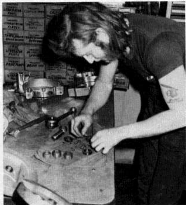
Medicine Man Bob Roach selects oversize rollers to obtain .0005 to .0015 clearance for both rod and main bearings.
