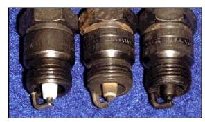
any fuel that has ethanol in it. (Ethanol is largely made up of hydrocarbons and as such it makes plug reading almost impossible due to the high carbon deposits that remain on the plug).
