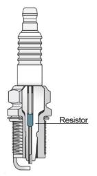
As a spark jumps off the centre electrode, some electrons move with it resulting in electrode wear which is normal. While high voltage is good, high amperage is not, more amperage results in more wear. Resistors reduce some of the current flow (amps) as the voltage moves through the plug. This has the benefit of increasing electrode life especially in HEI and CDI systems.
